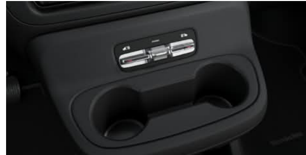
Electrical operation of sliding doors
