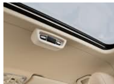
TEMPMATIC climate control at rear
